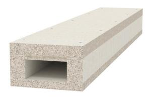
Fire protection duct made from water and frost-proof fibreglass lightweight concrete of building material class A1 according to EN 13501-1 for fireproof laying of cables in rescue and emergency routes, and for the maintenance of electrical functionality of safety-relevant systems. Classification I90 as I duct according to DIN 4102 Part 11 and classification E30 as E duct according to DIN 4102 Part 12
