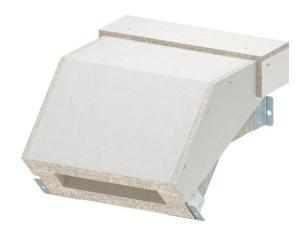
Falling vertical bend for PYROLINE® Con S fire protection duct, type BSKH09-K0521, consisting of fibreglass lightweight concrete which is resistant to water and frost for the creation of vertical changes of direction (45°) of the duct. Mounted connectors ensure quick mounting in situ, whilst loosely placed covers ensure quick inspection and reassignment.
