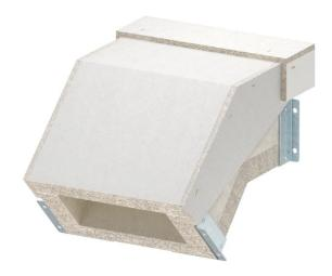
Falling vertical bend for PYROLINE® Con S fire protection duct, type BSKH09-K1021, consisting of fibreglass lightweight concrete which is resistant to water and frost for the creation of vertical changes of direction (45°) of the duct. Mounted connectors ensure quick mounting in situ, whilst loosely placed covers ensure quick inspection and reassignment.
