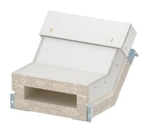
Rising vertical bend for PYROLINE® Con S fire protection duct, type BSKH09-K0521, consisting of fibreglass lightweight concrete which is resistant to water and frost for the creation of vertical changes of direction (45°) of the duct. Mounted connectors ensure quick mounting in situ, whilst loosely placed covers ensure quick inspection and reassignment.
