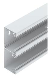
GS device installation trunking for mounting on the wall or on fastening panels. The GS device installation trunking possesses self-contacting locking straps to accept a sheet steel partition. The equipotential bonding between the trunking bases takes place using the trunking coupler. The protective measure and the equipotential bonding is guaranteed between the cover and the base by the self-contacting trunking cover. The real system opening is 76.5 mm. The cover must be ordered separately.
