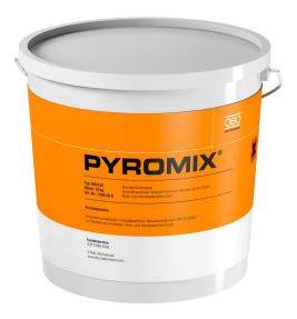
Mortar to create cable and combination insulation in solid walls and ceilings. Suitable for pumping, pressing and for manual installation. Adding approx. 3 litres of water to 10 kg of dry mortar produces about 10 litres of workable compound. For interior application.
