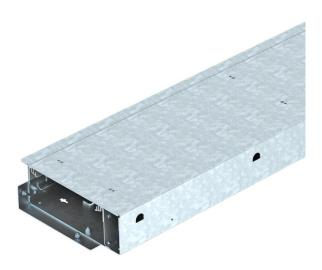
Ready-to-mount trunking unit for cable routing and device installation, consisting of a trunking base with two blanking covers. The scope of delivery contains two lid butt seals and one connector. For height adjustment, six height adjustment units are required. Load capacity up to a maximum of 5 kN. The trunking unit can be supplemented with an adjustable floor covering contact profile for screed limitation in areas of door frames and in front of radiator niches.
