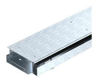
Ready-to-mount trunking unit for cable routing and device installation, consisting of a trunking base with two covers and a height-adjustable brush bar. The scope of delivery contains two lid butt seals and one connector. For height adjustment, six height adjustment units are required. Load capacity up to a maximum of 5 kN. The trunking unit can be supplemented with an adjustable covering contact profile for screed limitation in areas of door soffits and in front of radiator alcoves.
