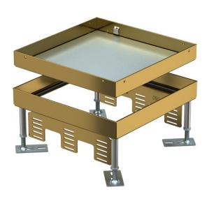
"Blank" height-adjustable cassette for the creation of an inspection opening of nominal size 4. Installation of devices in duct systems, raised and cavity floors in interior dry or wet-care floors. Only suitable for smooth floor coverings. For the installation of three UT4 universal supports for nine single devices with support ring/support clamp or 12 Modul 45® devices. 3 APMT5 cover plates can be installed.
