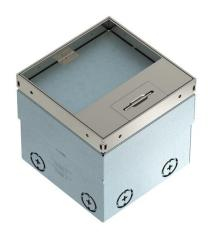
Square floor socket for use in dry-care cavity and screed floors in indoor areas. Installation housing with pre-marked insertion openings for pipes (M20/M25). Cover adjustable to top edge of floor covering using four height-adjustment supports. The minimum installation depth is 110 mm, the height-adjustment range is +25 mm
