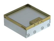
Square floor box for use in dry-cleaned cavity and screed floors in indoor areas. Installation housing with pre-marked insertion openings for pipes (M25). With three UT4 universal supports and two double sockets. Cover adjustable to top edge of floor covering using four height-adjustment supports. The minimum installation depth is 95 mm, the height-adjustment range + 30 mm.
